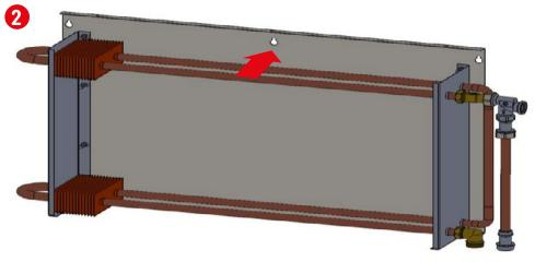
Fix the rear panel along with the attached exchanger to the wall by means of bolts and rawlplugs supplied in the kit, at the places indicated in picture.
