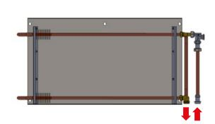
After fitting the rear panel, connect the supplying system shown in picture, tightening the nuts which can be found on the supply and return ports. In order to connect the heating device to the system, the nuts must be countered.
