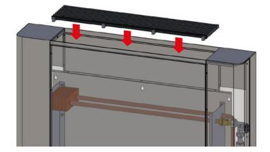
After the casing is placed with the panel and with the exchanger, install the casing with screws in the designated places shown in figure 6 by means of the screws supplied with the heater. The number of the fixing points may vary depending on the heater.
