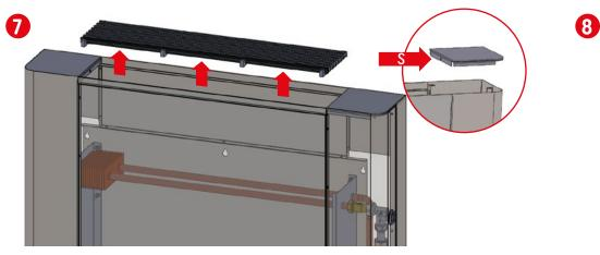
After the heater is connected to the system, vent it. For this purpose, remove the grate, and then disassemble the masking element, located on the valve side, by unscrewing the **S** screw and pulling the masking element out of the casing.
