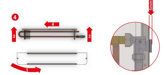
In the next step, install the casing in accordance with the diagram presented in picture, turning it, so that the valve is in the centre of the casing, and then level the casing with the rear panel. After placing and levelling the casing and the exchanger, the valve should protrude from the casing by approximately 5 mm.
