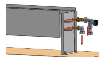
Then, connect hydraulically the heater with the central heating system. It is important to make sure that the connector pipes have been properly countered.
