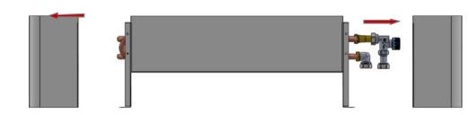
After removing the aforementioned elements, remove the covers of the legs (Fig. 4) and place the heater in its installation place.
