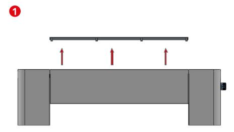
After taking the heater out of its packaging, in the first place, remove the decorative grate.
