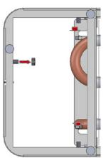
Next unscrew the masking elements along with the fixing covers. To do this, unscrew the lid and the pad under the masking frame.
