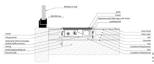
The example of VKN fan assisted heater assembly
