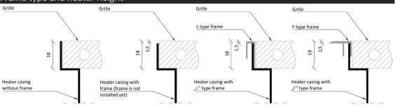
The height of the casing edge depends of the frame type. It is recommended to order frame together with heater or inform manufacturer about planned frame installation on later stage.
