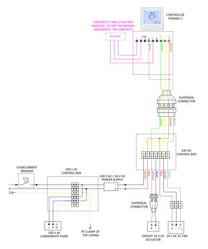
NOTE: Only properly skilled and trained personnel, holding licenses and observing applicable standards can install electric connections. Power can only be switched back on when the correctness of the whole wiring was checked and approved. Due to use of safe low voltage fans the heaters can only be powered by 24 V DC voltage. It is prohibited to connect the heaters directly to 230 V AC power grid.
