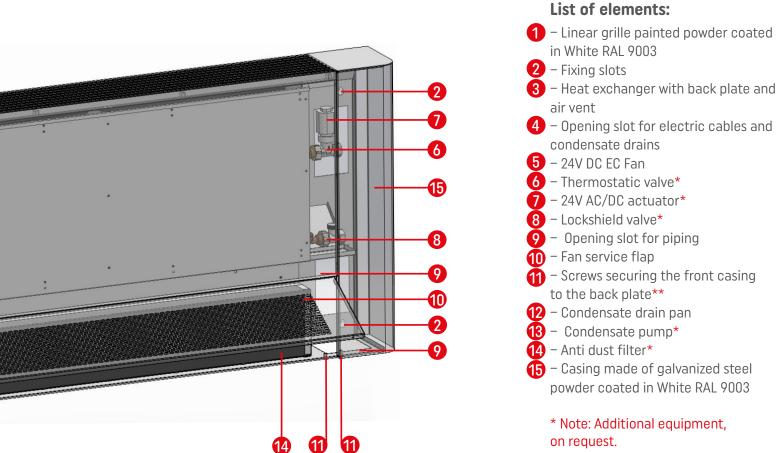
15 – Casing made of galvanized steel powder coated in White RAL 9003 \* Note: Additional equipment, \*\* Note: The number of mounting
